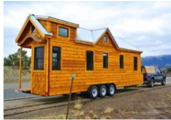
Tiny House on Wheels Complies with existing code for trailers and RVs.
